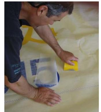
I recommend removing and installing the numbers and insignia one side at a time – it alleviates having to flip and roll the sail.
