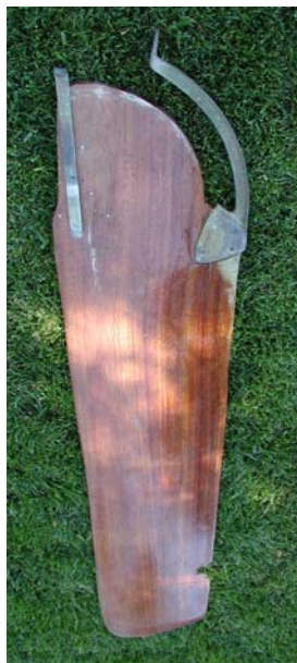
1 st generation classic Lido 14 centerboard with riveted on bronze arm and press fit hangers
