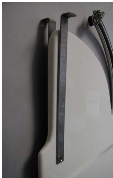
3 rd generation classic Lido 14 centerboard with stainless steel arm and removable stainless steel hangers
