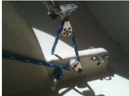
Centerboard uphaul rigged for 2:1 purchase
